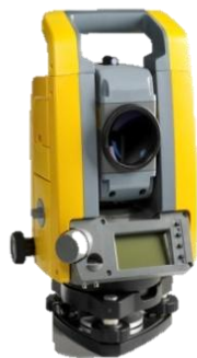
Robotic Total station
