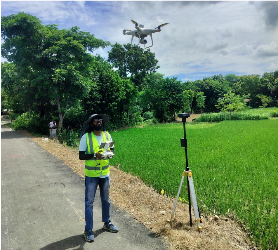
Figure: Survey with DJI Phantom version 2 RTK Drone
